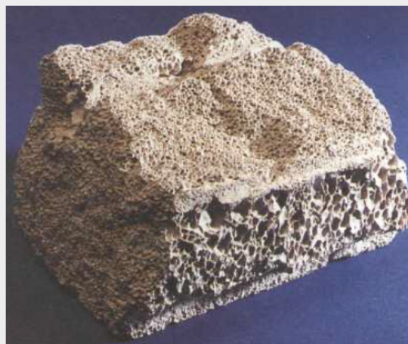
● Figure 2 A lump sample of AAC [1]
